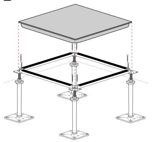
Each tile is supported by a steel structure-pedestal and screwed stringers with different heights so it is possible to access to the space under the floor, that can be used for electric installations, water pipelines, air conditioning,
